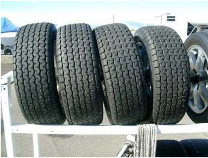
Lot's of tread to channel water through the tire. Saturday's rain tires: Hoosier Dirt Stockers.
