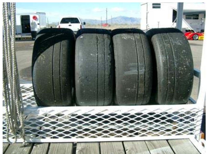
Lots of surface area for dry traction. Sunday's dry tires: Kumho Ecsta V710.
