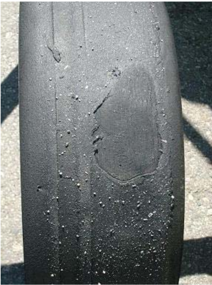
Delaminated Front Tire from heavy braking.
