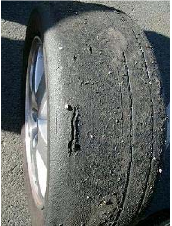
Front tires that have started to delaminate.
